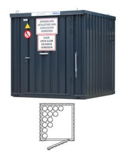
Hiltra F60 gas bottle depot model BSG 2 210220364 External dimensions 2090 x 2170 x 2240 mm **WxDxH** Dimensions internal 1810 x 1800 x 1925 mm BxDxH 49x 50 liter standard cylinder Capacity Weight approx. 985 kg Door Lockable single door B=1300 mm with emergency unlocking mechanism
